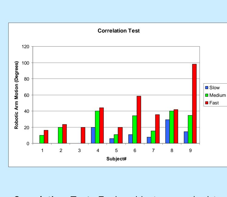
Correlation Test: Each subject was asked to flex their biceps in three different paces slow, medium and fast. The starting point was from rest at 0 degrees to the completely flexed position of approximately 150 degrees. The corresponding robotic arm movement was recorded and tabulated.
