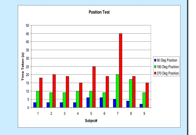
Position Test: Users were asked to move the robotic arm to three different positions at 90, 180 and 270 degrees. The ease with which each user was able move the robotic arm with biceps contractions is reflected on the time it took them to move to the designated positions.
